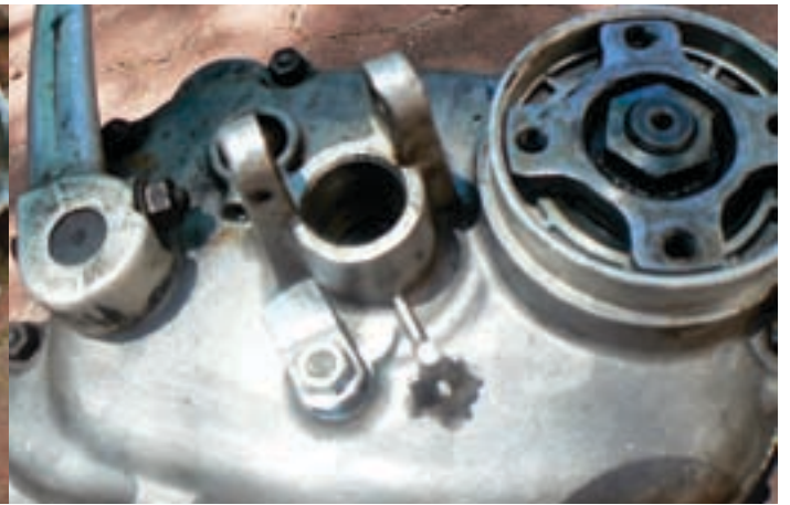
This similar repair to the idler gear shaft was done to a spare 4-speed I purchased a couple of years ago. While looking a bit rougher, I'm sure it did the job of securing the shaft.
